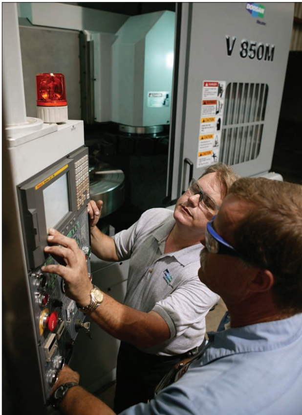
Employees program the controls of 101 Pipe & Casing's Doosan vertical turret lathe, which uses computer numerical control technology to manufacture seamless pump column couplings.
