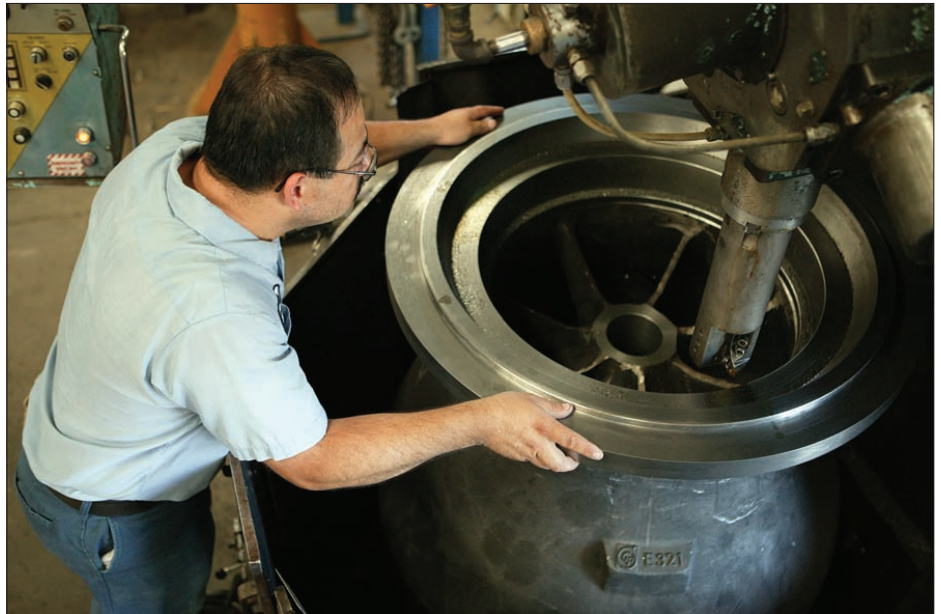
Based on the customer's specifications, a 101 Pipe & Casing employee tends to the machining of a pump bowl. The company currently has a customer base of 1500.
